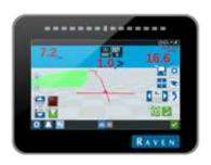
This field computer acts as an accessory for the Raven computerized kit sold from BioBased Spray Systems. It allows for the tracking and recording of the gallons of material applied over the total area. This systems also utilizes a GPS smart antenna to monitoring and trace precisely where product is applied.
